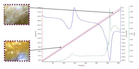
Left: Results from TASC compliment DSC data, and often show a more precise shoulder to the phase transition. Right: View all LINK's measured parameters on one graph and see how DSC and TASC data evolve with time and temperature. LINK captures images as the experiment progresses which is shown alongside temperature data.
